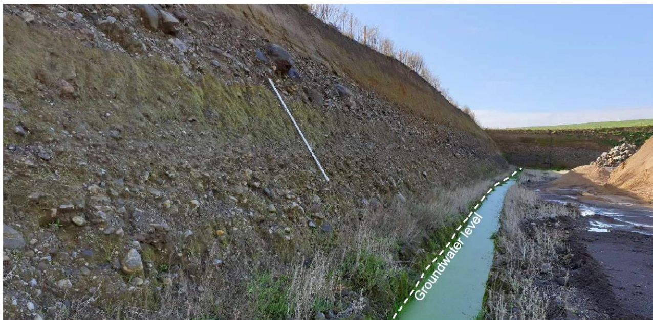
Figure 5: Ngaere Formation (tight) alluvium exposed in northwest face. White stick is 2.4 metres long. Pit floor is just above the groundwater level exposed in the ring drain.
