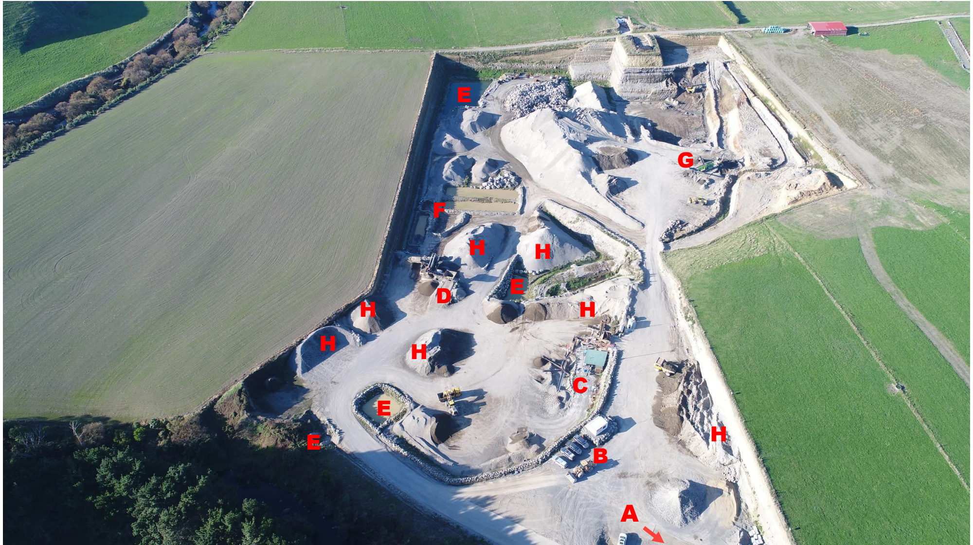
Figure 7: Site Layout. A: Visitor and machinery parking. B: Site office and staff parking. C: Crushing plant. D: Wash processing plant. E: Stormwater ponds (x3). F: Washwater ponds. G: Screening machine. H: Stockpiles
