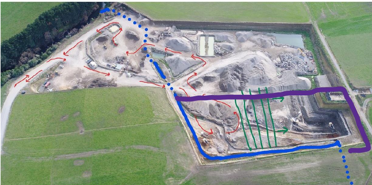
Figure 6: Red arrows shows truck movements. Blue shows the flow of the open and piped tributary.
