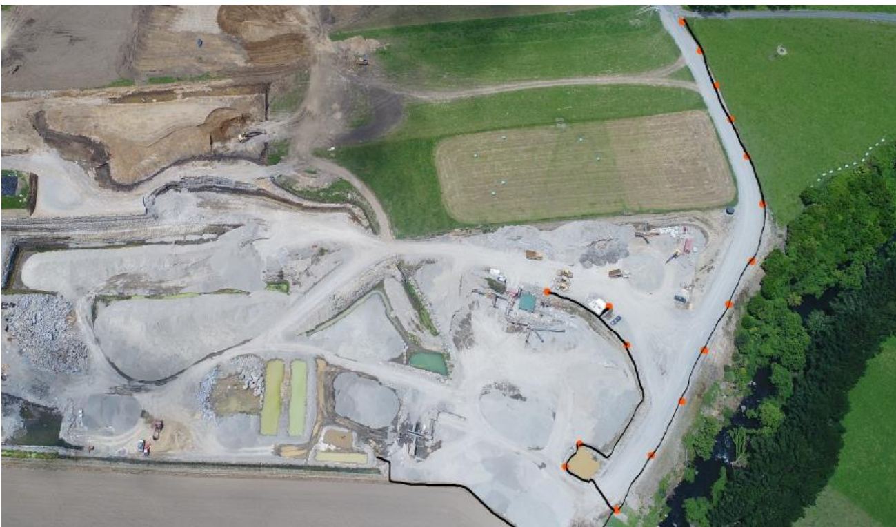
Figure 28: Red dots and black line indicate the location of the sprinkler system
