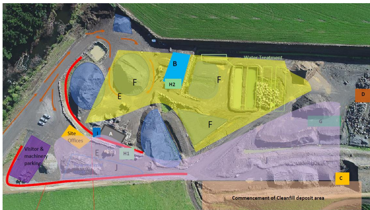
Figure 8: Site layout for equipment. A- Crushing plant and generator. B- Wash plant processing. C - Digger (Volvo EC300) and excavator (30T). D - Excavator (36T). E/F - Processing stock pile areas. G - Screen machine. H - Fuel pumps. I - excavator (1.8T). J - area where dump trucks will be working.
