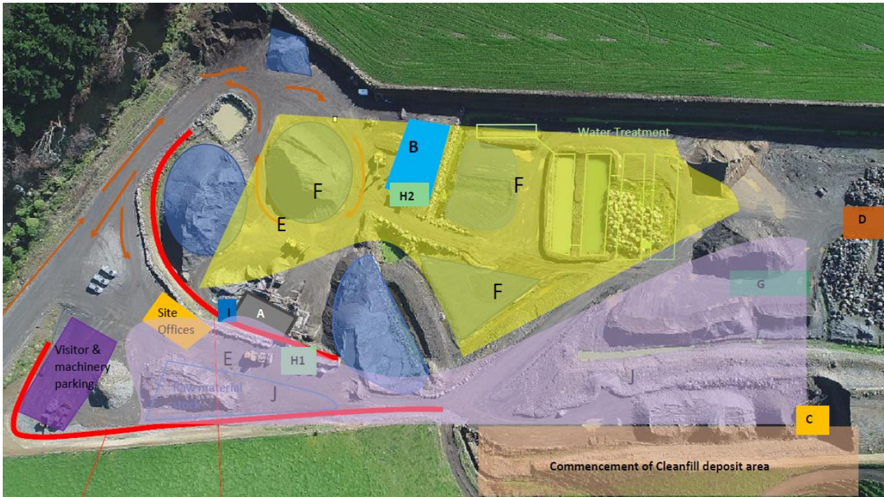
Figure 5: Site layout for equipment. A- Crushing plant and generator. B- Wash plant processing. C - Digger (Volvo EC300) and excavator (30T). D - Excavator (36T). E/F - Processing stock pile areas. G - Screen machine. H - Fuel pumps. I - excavator (1.8T). J - area where dump trucks will be working
