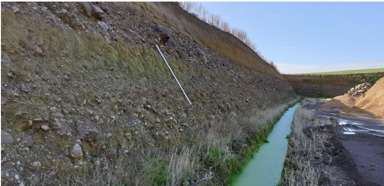
Photograph 1 Northwest face. White stick is 2.4 m long. Pit floor is just above the groundwater level exposed in the ring drain (Geosearch 15 May-19)
